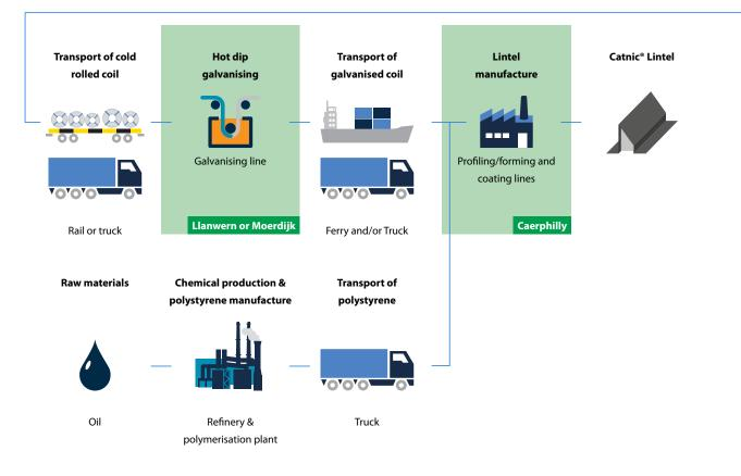
Process data for the manufacture of cold rolled coil at IJmuiden and hot dip galvanised coil at Llanwern was gathered as part of the latest worldsteel data collection. Process data was also gathered for the hot dip galvanising process at Moerdijk and for the lintel manufacturing process at Caerphilly.
