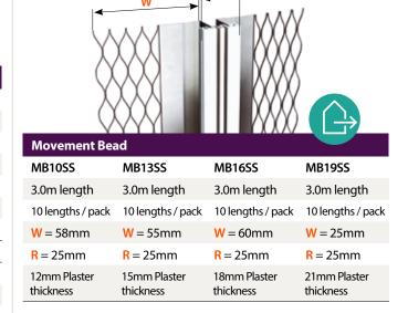
Quality: Manufactured from Stainless Steel to BS EN 10088-2-1.4016. All beads shown are manufactured in accordance with BS EN 13658-2:2005.
