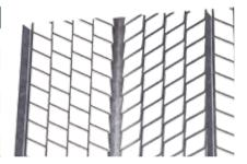
Quality: Catnic expanded Rib Lath is manufactured in accordance with BS EN 13658: 2005. Metal Lath - Definitions, Requirements, Test Methods. Part 1 for Internal Plastering. Part 2 for External Plastering. The galvanised steel used in the manufacture of Rib Lath is in accordance with BS EN 10346: 2009 – DX51D+Z275. Where stainless steel is used it is in accordance with BS EN 10088-2-1.4301.
