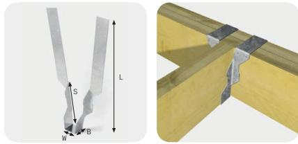
Medium-weight hanger suitable for joist depths up to 250mm, designed with 50mm strap legs, the longer length leg is suitable for face fixing or wrapped over supporting floor joists. Manufactured from 1.2mm thick hot dipped galvanised steel, Z275 coating to BS EN 10346: 2015. Designed with a 50mm bearing surface, hangers must be secured with 30 x 3.75mm sheredised square twist nails, through all individual pre-punched holes.
