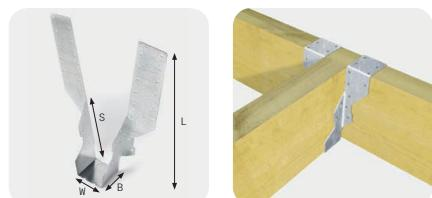
Lightweight hanger suitable for joist depths of 150 to 250mm and face fixing, designed with 50mm wide strap legs with increased nail spacing\*. Manufactured from 0.9mm thick hot dipped galvanised steel, Z275 coating to BS EN 10346: 2015. Designed with a 50mm bearing surface, hangers must be secured with 30 x 3.75mm sheradised square twist nails, through all individual pre-punched holes.
