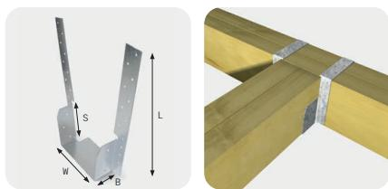
Medium-weight hanger suitable for joist depths up to 250mm, designed with 40mm wide strap legs and location tab on hanger base for quick and accurate alignment. Manufactured from 1.2mm thick hot dipped galvanised steel, Z275 coating to BS EN 10346: 2015. Designed with a 50mm bearing surface, hangers must be secured with 30 x 3.75mm sheredised square twist nails, through all individual pre-punched holes.
