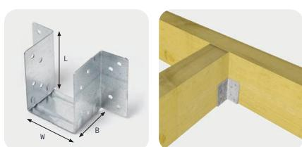
A lightweight hanger suitable for joist depths up to 100mm, ideal for trimming around ceiling hatches, and similar light duty applications. Manufactured from 0.8mm thick hot dipped galvanised steel, Z275 coating to BS EN 10346: 2015. Designed with a 40mm bearing surface, hangers must be secured with 30 x 3.75mm sheredised square twist nails, through all pre-punched holes.
