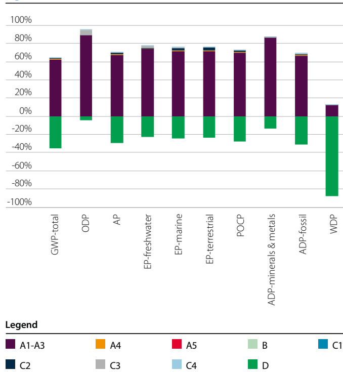
Figure 4 LCA results for Catnic® CG90/1001500 lintel
